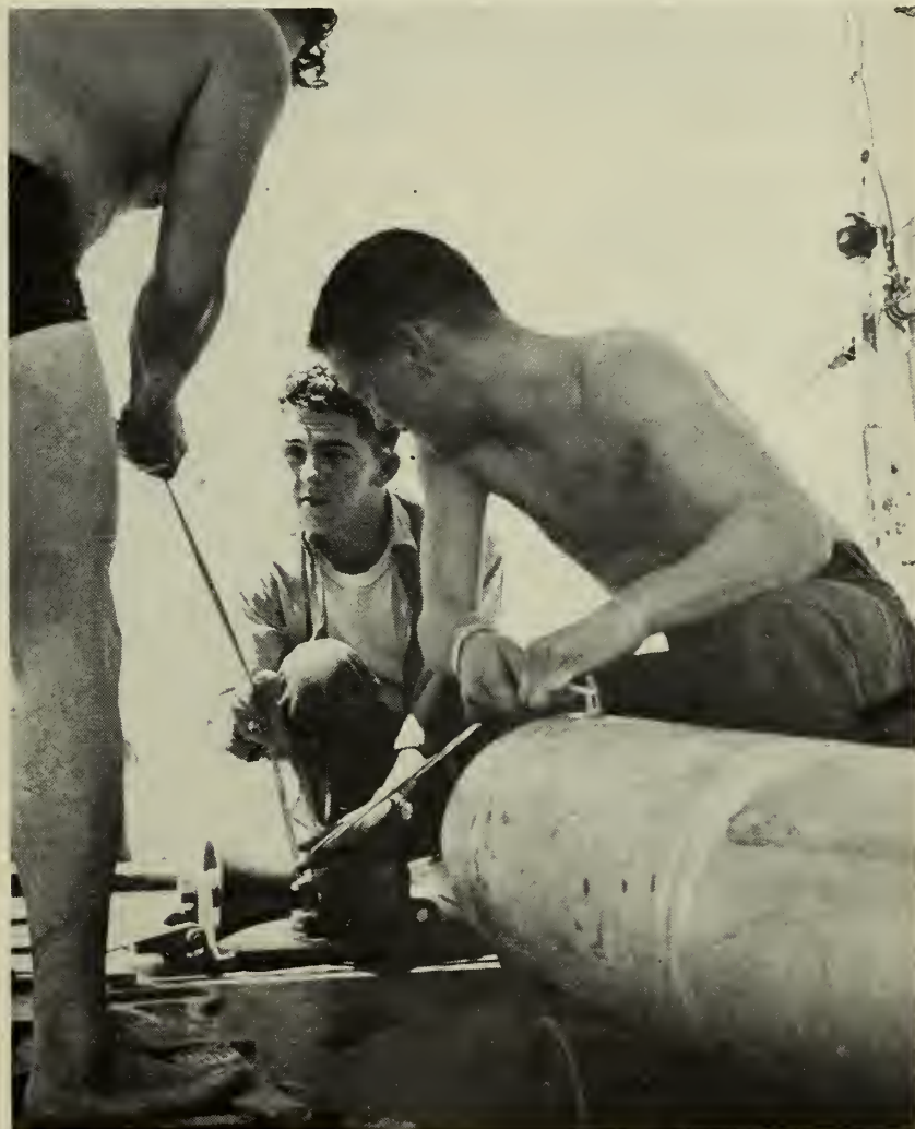
ALL ABOARD—Torpedo is hooked (above) and pulled up ramp at after end.
